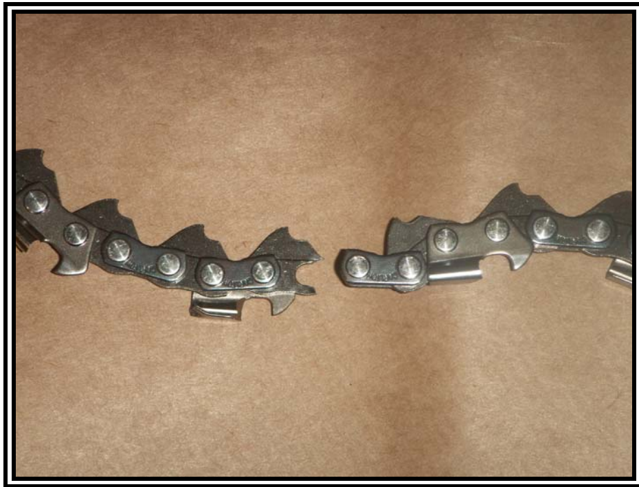
Figure 3: Tensile Failure Location
